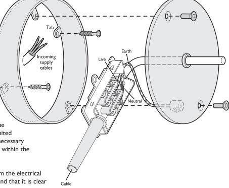
Carefully conceal the connector block and any spare cable within the wall/mounting cup and use two appropriate screws to secure the wall light onto the surface. Ensure that the screws do not interfere with the mains cable.
