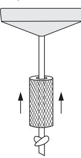
3 Take the smaller part of the splitter, feed one end of the other piece of cord through the flat end so that it comes through the other side.
