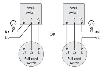
You need to connect your new switch to the circuit in exactly the same way as the one that it is replacing. This product must be installed in accordance with local building regulations.
