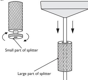
2 Tie a knot at the end of the cord and pull the larger part of the splitter back over the knot to secure it in place.
