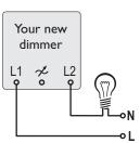
Your dimmer has two terminals labelled L1 and L2. You need to connect the live mains feed to one of the two terminals and the cable from the lamp(s) to the other terminal (it's not important which way round). The earth connection is not shown in this diagram but it is essential.
