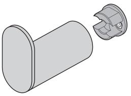
10 Use the supplied Allen key to tighten the grub screw(s) so that the accessory becomes securely locked onto the inner lug(s).
