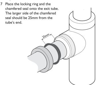
8 Insert the tube into the bottle trap's exit hole so that the seal seats evenly on the mouth of the exit hole. Semitighten the locking ring to hold the tube in place.
