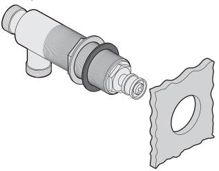
8 Place the finish ring onto the protruding threaded section and tighten it so that the control body is held tightly in place, with its outlet pipe facing downwards.
