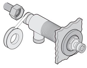
10 Place a single wrap of PTFE tape around the thread of the outlet on the underside of the control body - but ensure that the tape does not go onto the flat face of the outlet. Attach one of the braided link pipes (it's not important which one) to the outlet and tighten its nut.
