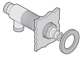
9 Place a single wrap of PTFE tape around the thread of the inlet at the rear of the control body - but ensure that the tape does not go onto the flat face of the inlet. Attach the cold water supply pipe to the inlet and tighten its nut.
