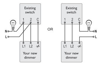
You need to connect your new dimmer to the circuit in exactly the same way as the switch that it is replacing. Note: You can only replace one of the existing switches in a 2-way installation, dimmers cannot be used at both ends. This product must be installed in accordance with local building regulations. IMPORTANT: If you are in any doubt, STOP and seek professional help. Do not proceed unless you are sure.
