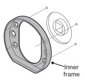
4 Mark the mounting holes that you will use. The inner frame has six holes; you do not usually need to use all of them, however, more fixings can help to make the handles more secure. 5 Carefully drill small pilot holes for the screws and mount the inner frame in place using the supplied screws.
