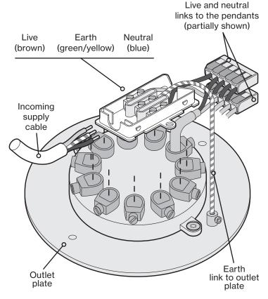
Note: It is not essential to use the supplied rubber cable sheath on the connector box.
