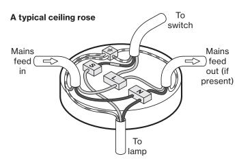
To recreate loop-in connections: Remove the supplied connector block. Using the labelled cables as discussed left, you now need to recreate the loop-in circuit links that existed in the original rose, using suitable connectors (that are rated and insulated for 240VAC use) - such as Wago® terminal blocks (part number 221-413)). You will need four of these connectors to form the live, neutral, switched live and earth connection groups.
