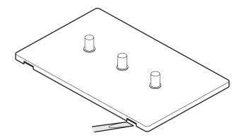
3 Lift the plate up and away from the body of the switch/dimmer.
