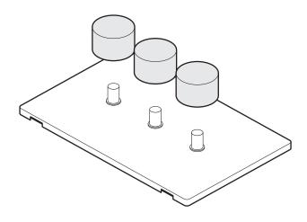
2 On the underside of the switch plate insert a small flat tool into one of the base slots and carefully prise up the plate.
